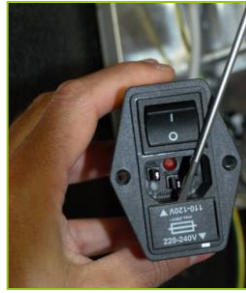
Figure 11 Illustration of the fuse door opening operation
